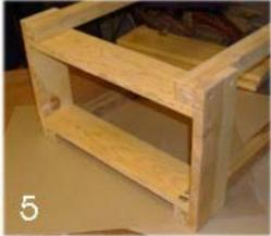
Turn this entire assembly over, lay the second 18" piece in place, and drill pilots at both ends (see illus. 5). (Note: because the height is restricted, the pilots will drill both from the outside of the frame and inward toward the corner at the same time.) Remove the 18" piece, make countersinks, and put glue in the joint. Again, set the first screw at each end part-way, drive the second, then drive the first.
