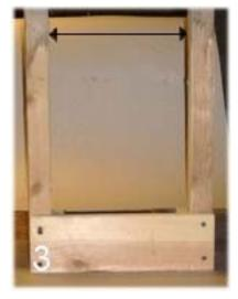
Assemble the other end, the 12" piece and the legs: make its angles match the first ends's angles by standing both ends upside down and touching the legs together before setting the "second" screws.
