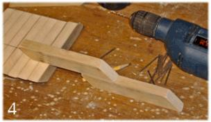
The brackets assemble face-down on the table (illus. 4). Line up the blunt end of the first piece at the line on the "front" of the second piece and drill a pilot hole slightly undersized for a six-penny finishing nail (two-inches long) through/into both pieces of wood. The hole should best not come out the front of the lower piece.
