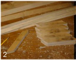
Need some thin plywood for the cross-pieces (1/4 or thinner: this is Asian cratewood, though I've generally used the ripped and split thickness of a 2x4 to make 3/16 by about 3/4 inch strips) (illus. 2). Need some maybe 3/8 inch thick pieces 1 1/2 inch wide for the wall-brackets (the side of a 2x4 works well: it's already "eased"). The sample has one pointed-end cut blunt (a very little bit).
