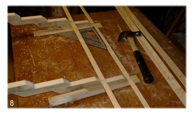
NOTE: As shown, the six plywood strips require five bracket pieces, but the bracket pieces will stand between the ribbons. If the strips are tacked on the faces of the bracket pieces, just at the top of their vertical faces, this six-row rack would need one more bracket-piece, but could be made to "hide" the bracket-piece faces.
