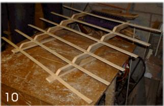
Drill holes for wall-mounting screws in the upper ends of the 1 1/2 inch strips, and slightly countersink the faces (illus. 10).
