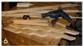
With the brackets assembled (illus. 6), mark the 1 1/2 inch wide bits of 2x4 edge that will be the wall-mounts, pre-drill them for three-penny nails, glue the surfaces, and nail-up.
