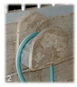
For both holders, plywood dimensions are within half-an-inch of each other, so here are the plywood measures for the "larger" one: Wall-mount plywood (as is the core) is eight inches wide (illus. 2), and is 9 1/2 inches high. The front plywood is ten inches wide by eight inches high (illus. 3). I don't know what I'd used to set the "curve" for the top of its wall plywood (not much, it looks like), but probably the bottom of a muck bucket for the front.
