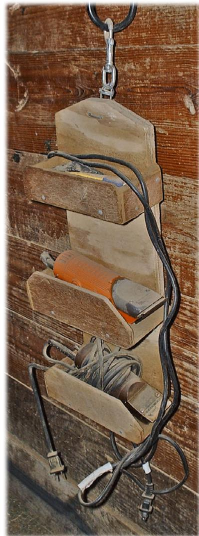
Shorter pieces of this thin plywood make back ends to these trays, keeping the extended cord from pulling the clipper motors off the caddy. Four inches of open space exist between each of the clipper trays.
