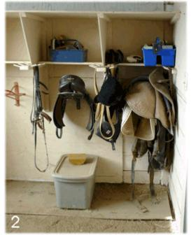
I glued and screwed 2x2 to two of the triangle-sides, as shown (illus. 2). I took 2x4 pieces 23-inches long, made an opening half-an-inch wide and out about thirteen inches from what would be the wall (the opening to slip over the plywood, and its sides to support shelves) (illus. 2). I glued and nailed the 2x4 pieces (I'd round-over routed the edges) eighteen inches from the top of the plywood. I see that I had slightly notched the plywood to more nicely accept the 2x4 pieces.
