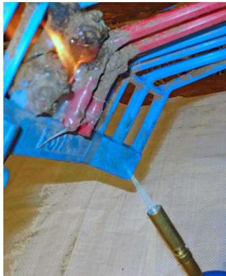
If a replacement tine snaps, the only way I've found to remove the glue is to carefully soften it with a small propane torch.
